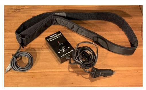
The Kendrick dew remover system is designed to **eliminate dew from telescope optics** by keeping the optics slightly warmer than ambient, or above the dew point. Power is applied from a dew controller via flexible dew heaters, usually wrapped around the telescope tube, near to the cell housing the optics.
